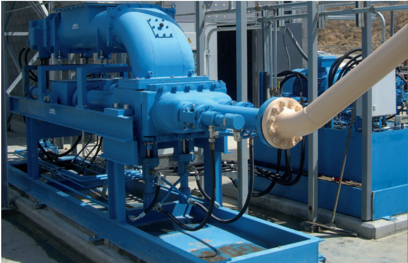
ABEL SH with double screw feeder for transfer of dewatered sewage sludges
